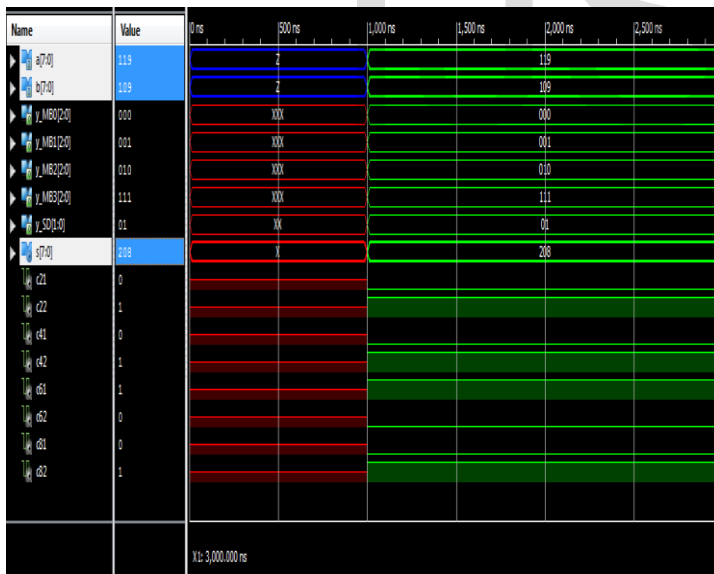
Fig6: Simulation results for X=119, and Y =109 those in decimal form and their related partial products
